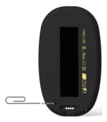
2. Put the Vario LS into "fail safe" mode: keep the Power/Menu button pressed, while pressing the reset button. Keep the Power/Menu button pressed untill a counter is displayed on the screen. After the counter ends the Vario LS should display "SAFE" text on the graphic area. The firmware can now be installed by using manual update (chapter 4), or, exit the "fail safe mode", pressing the reset button again.
