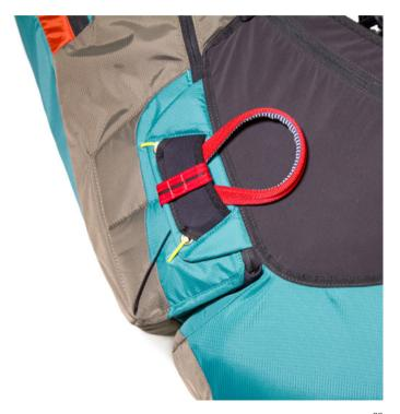
when not sitting in the harness as for flight. The release procedure must take place in the flying position, without hindrance, and in accordance with the requirements of this manual. The force required to release the reserve must not be less than 4 daN and not more than 7 daN. If in doubt you should contact a qualified person or your ADVANCE dealer.
